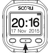
4. Press OK. The initial time is blinking, meaning it can be modified.
