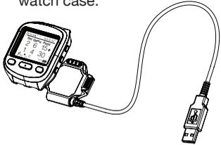
2. Plug the USB connector of the cradle charger to the PC.
