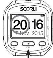
5. Press the A and B buttons to adjust the time field. Press OK to save and move to the next field
